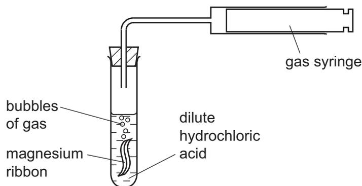
The total volume of gas produced is measured.
